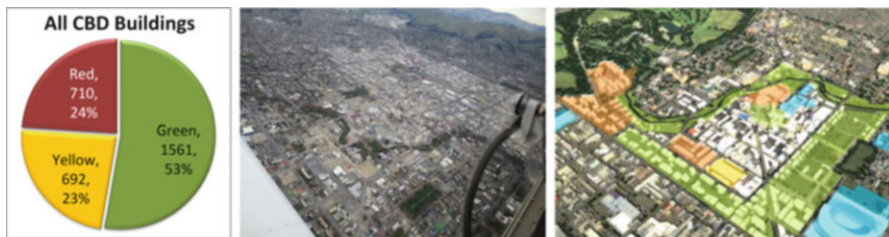
Fig. 13.4 Left : distribution of buildings tagging statistics in the CBD (updated to 12 June 2011, Kam et al. 2011); Centre : Aerial view of CBD with entire lots demolished and “cleaned up” (Photo courtesy of Kam Weng and Umut Akguzel); Right : CERA Blueprint
