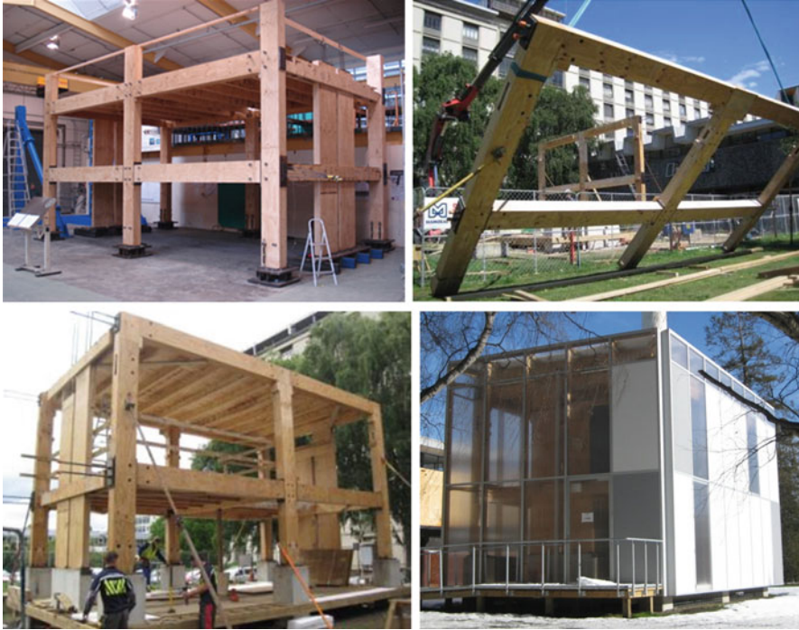
Fig. 13.29 From laboratory specimen to office building: 3D Test Specimen tested in the lab (Newcombe et al. 2010), demounted and reconstructed (Smith et al. 2011) on UC campus as EXPAN/STIC office
