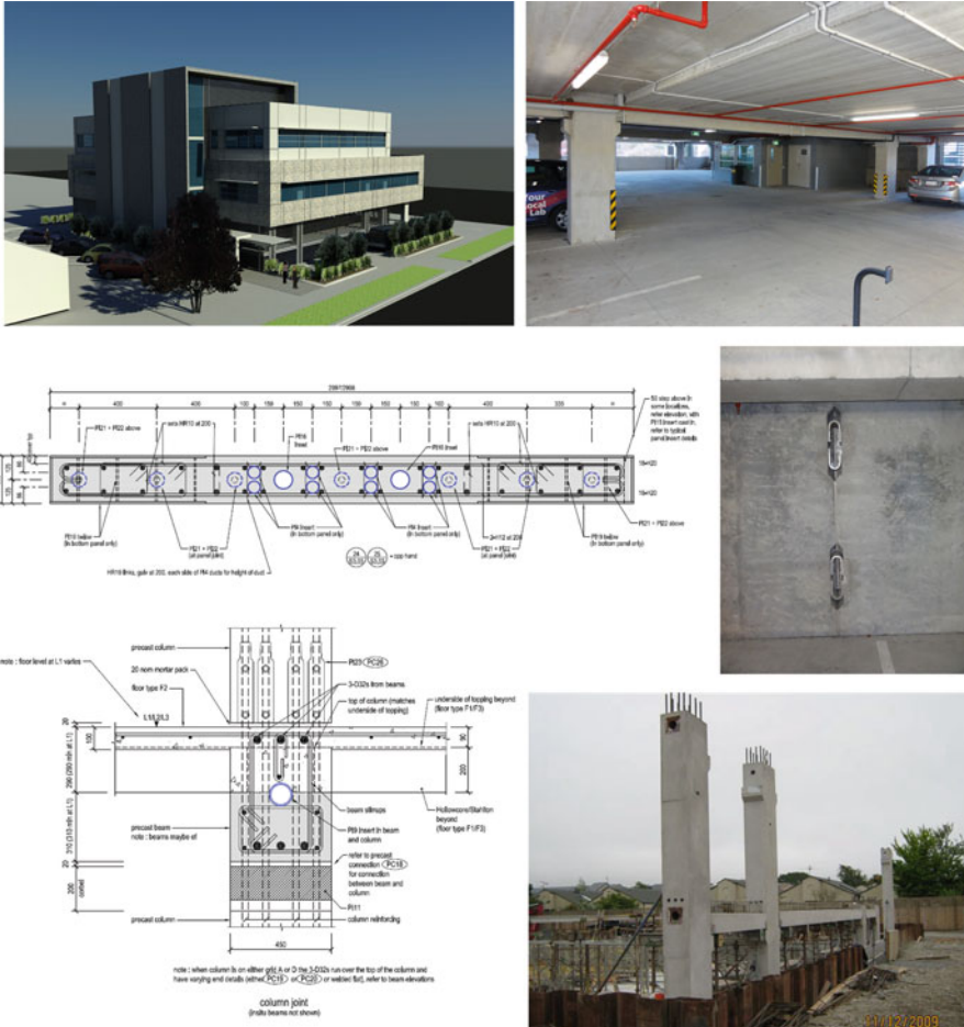
Fig. 13.25 Southern Cross Hospital Endoscopy Building, Christchurch Rendering, construction of the frame, details of beams, walls and U-shape Flexural Plate dissipaters (Structural Engineers: Structex Metro, Pampanin et al. 2011)
